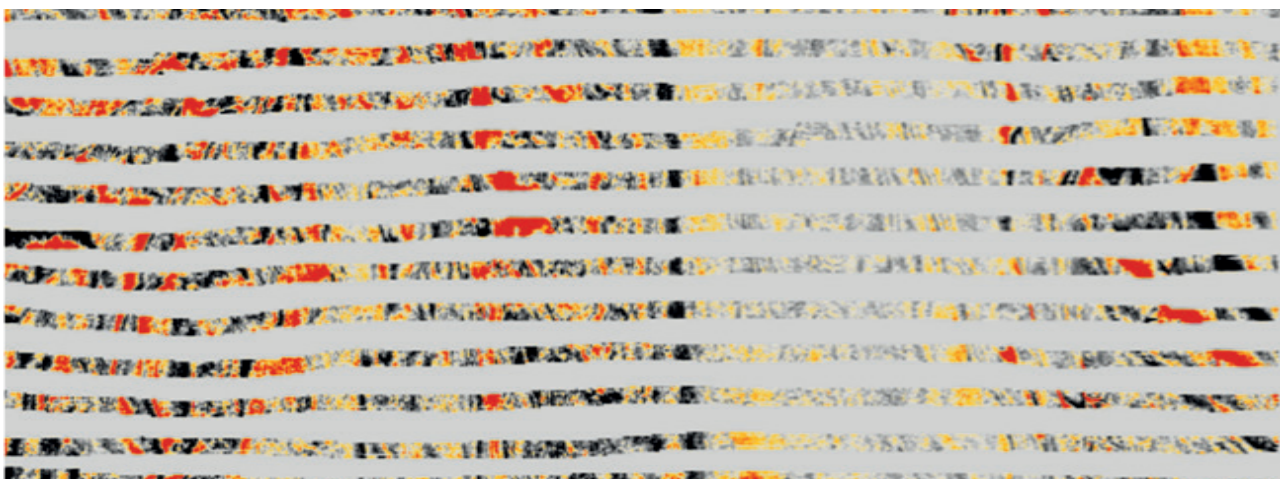
Time slice through a near offset, marine dataset showing holes in the coverage caused by variable currents.
