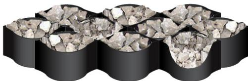
A 125mm Depth of well compacted, non-frost susceptible Type 3 granular sub-base to SHW clause 805 or 4/40, 4/20 graded crushed concrete aggregate to BSEN 12620 or locally available secondary or recycled aggregates which comply with the requirements of the specifications for Highway works for sub-bases in conjunction with a 100mm deep 'Cellweb<sup>™</sup>' or similar standard cellular confinement blanket and a 25mm surcharge.
