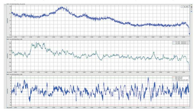
Quality checks on the source array performance are generated during acquisition. The array strengths should track one another closely. The values displayed are obtained from the target RMS values calculated on the centre streamers. The second graph plots the percentage difference between the two source arrays.
