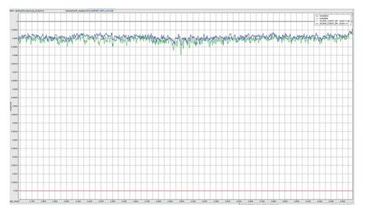
The cross correlation values between the reference far field signature and the real time calculated far field signature are displayed in a graphical format as the line progresses. This display can highlight gun substitutions, changes in source geometry and source malfunctions.
