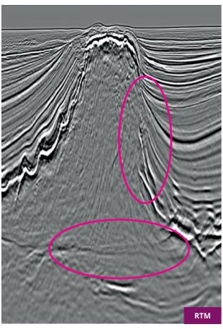
The Shearwater RTM is our most advanced depth imaging method. It is suited to geology with rapid or sudden lateral changes in velocity that cause significant distortion of the wavefront. Its use of the two-way wave equation allows clear imaging below the most complex overburdens. The input velocity models can also include small scale details.
