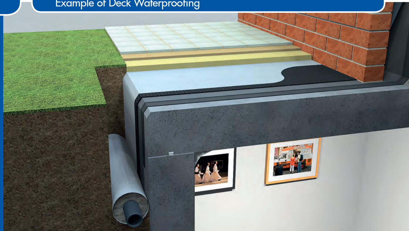
Newton inverted warm roof detail interfacing with the damp proof course and the internal System 500 Cavity Drain waterproofing
