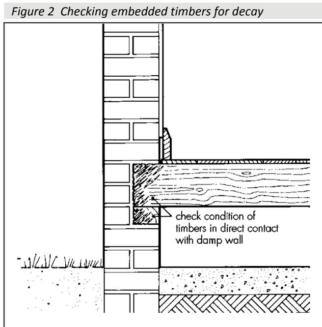
11.3 If damage is limited to the joist ends, the floors may be re-formed, using sleeper walls or joist-hangers, to isolate the timbers from the damp wall (see Figure 3).
