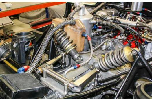
Rear suspension detail showing shock absorbers, coil springs and titanium anti-roll bar. *Author*
