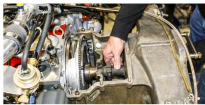
The splined power take-off between clutch and gearbox allows quick and easy clutch replacement in situ.
