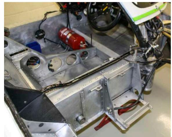
Monocoque of 956 114, repaired after the battery carrier was punched into the side at Brands Hatch in 1986.
