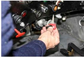
On 1987 factory cars, and standardised for 1998, the 962 had a purpose-designed door pull handle, utilising 928 latches and painted red to catch the attention of marshals.
