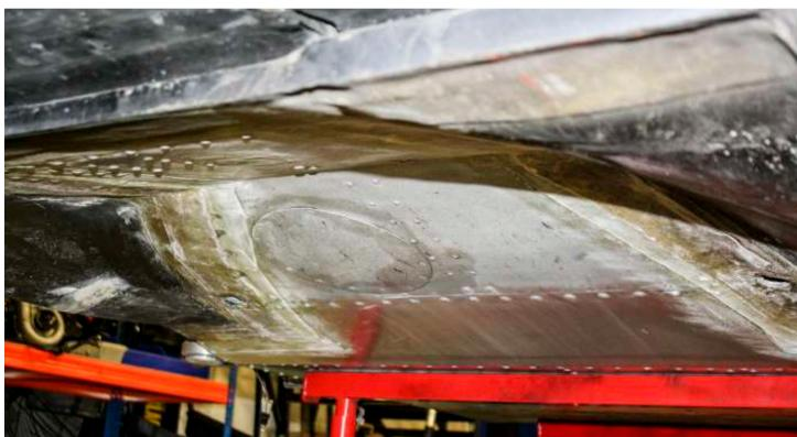
Cockpit and underfloor views of 956 114, showing the circular repair under the dash after Philippe Streiff ran over Aston Martin crash debris at Le Mans in 1984.
