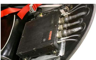
Used for the first time by the factory at Kyalami in 1982, the Bosch Motronic engine management system became standard wear on both factory and customer cars. This unit is a 1988 MP1.7.
