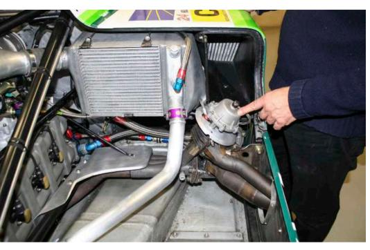
Detail of the turbocharger and intercooler, with stubby exhaust pipes exiting body side; these were vulnerable to side collisions.
