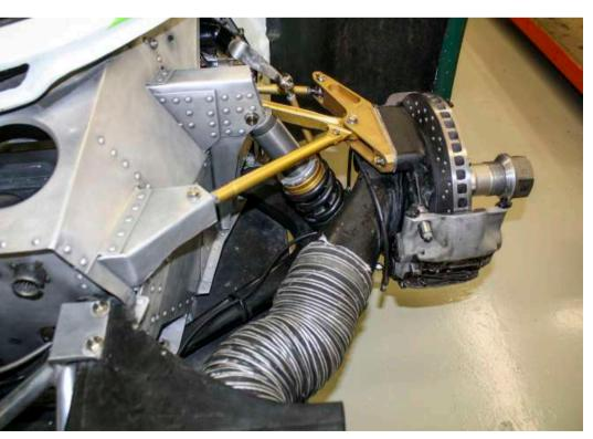
Front suspension with shock absorbers and coil springs now mounted; twin-caliper ventilated disc brakes require massive ducts for cool air. Author
