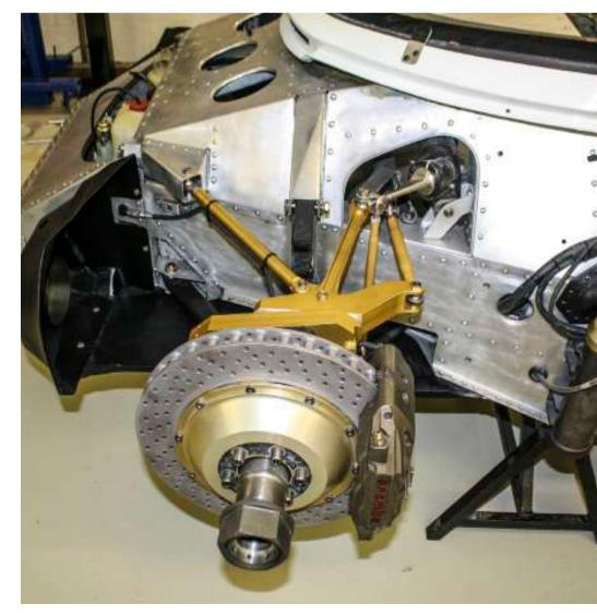
Comparison views of 956 114 (upper) and 962 007 (lower): the front suspension on a 962C is cranked forward to move the front axle centre line ahead of the pedal box.
