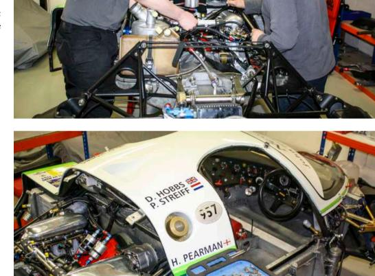
are working. All wiring looms are removed and thoroughly cleaned, and inspected for damage to wires and terminals. Then all is retaped to look as good as new.
