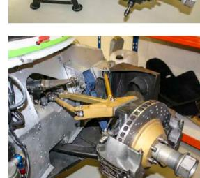
Driveshaft detail and Aeroquip oil-cooler piping to the gearbox; Porsche fabricated most components in-house, although others copied. Author
