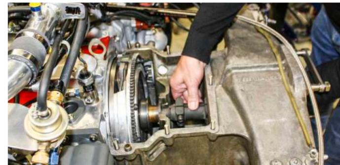
■ The splined power take-off between clutch and gearbox allows quick and easy clutch replacement in situ.
