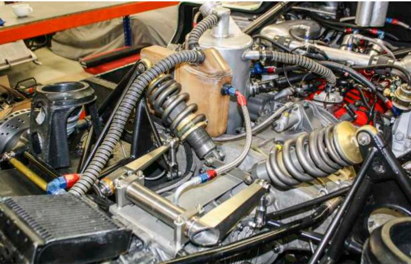
■ Rear suspension detail showing shock absorbers, coil springs and titanium anti-roll bar.
