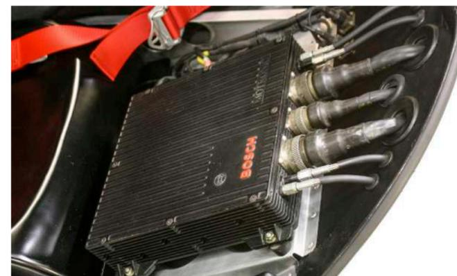
■ Used for the first time by the factory at Kyalami in 1982, the Bosch Motronic engine management system became standard wear on both factory and customer cars. This unit is a 1988 MP1.7.
