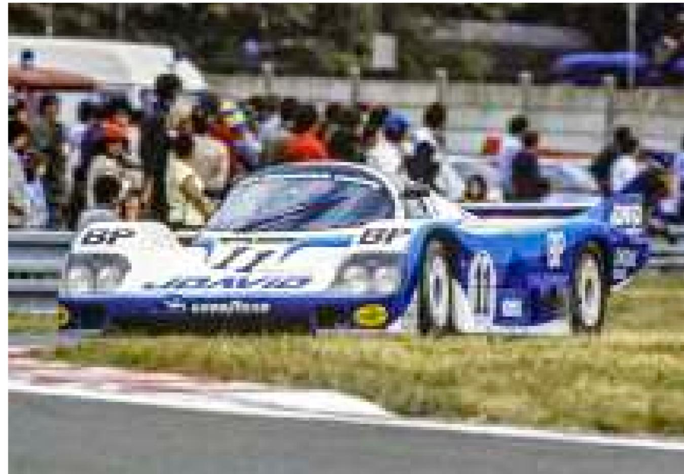
■ JFR's lead car, running in JDavid colours with Skoal Bandit decals, lay fourth behind the three factory Rothmans Porsches when its fuel pump drive broke at around midnight, stranding the car out on the circuit.
