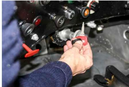
■ On 1987 factory cars, and standardised for 1998, the 962 had a purpose-designed door pull handle, utilising 928 latches and painted red to catch the attention of marshals.
