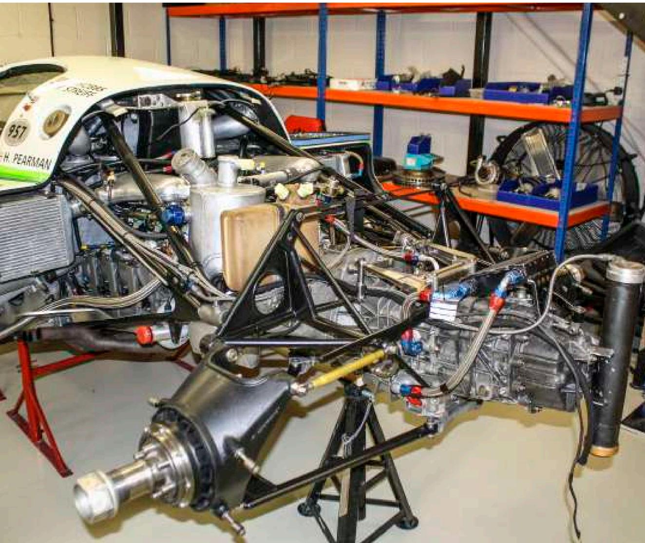
■ Rear suspension detail free of brake-cooling pipes; note upper/lower wishbones and rocker arms before shock absorbers and springs are fitted.
