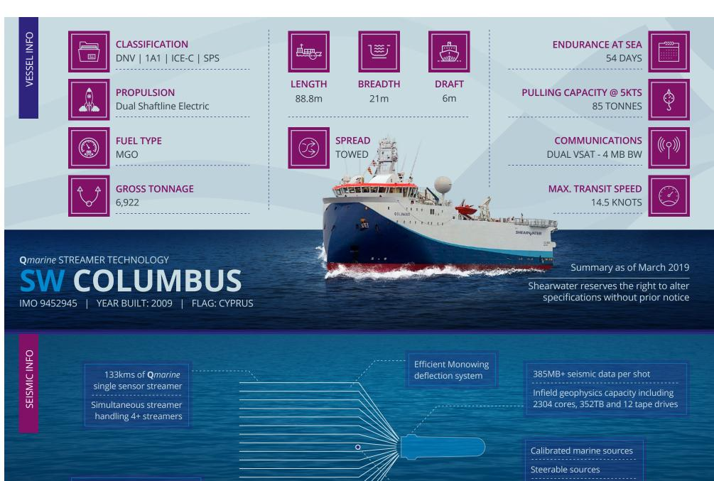
Steerable streamers (**Q***fins*) Integrated streamer acoustics TRINAV 6 positioning system
