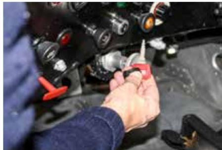
■ The 956 had a purpose-designed door pull handle, utilising 928 latches and painted red to catch the attention of marshals or rescue crews should the car be in trouble.
