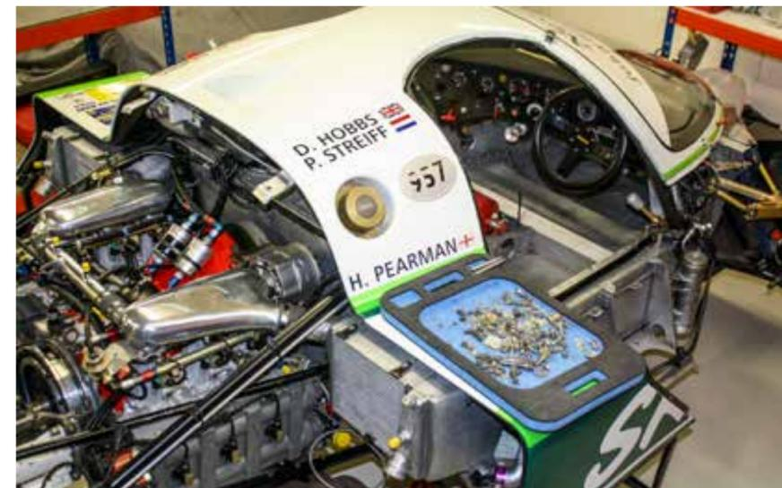
are working. All wiring looms are removed and thoroughly cleaned, and inspected for damage to wires and terminals. Then all is retaped to look as good as new.
