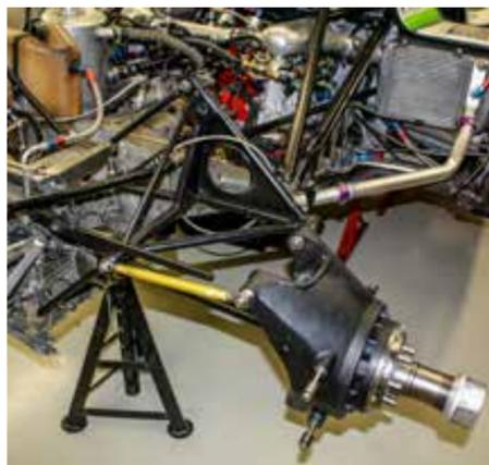
■ The front brakes use twin calipers to slow the car down from the high straight-line speeds achieved at Le Mans; note the all-important pad-retaining clips.
