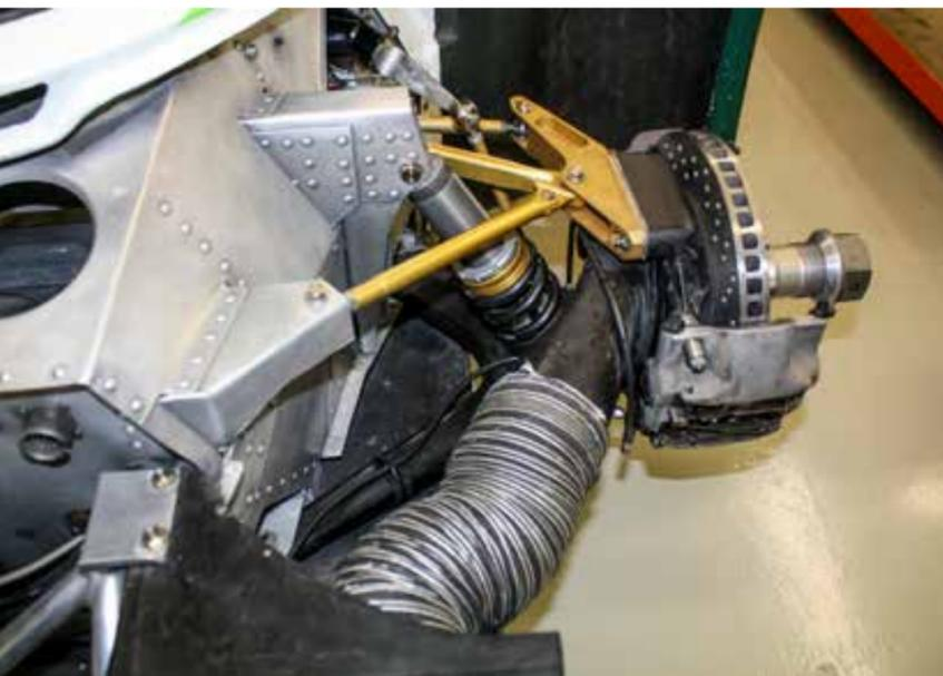
■ Front suspension with shock absorbers and coil springs now mounted; twin-caliper ventilated disc brakes require massive ducts for cool air.
