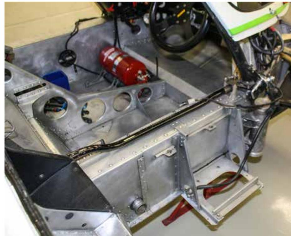
■ Monocoque of 956 114, repaired after the battery carrier was punched into the side at Brands Hatch in 1986.
