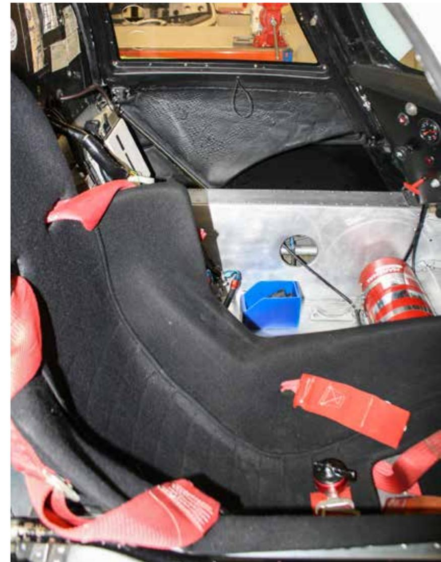
■ Deep driver's seat — all Group C Porsches were right-hand drive — has five-point safety harness; sportscars were, and remain, two-seaters by definition, even if only a dummy passenger seat was fitted.
