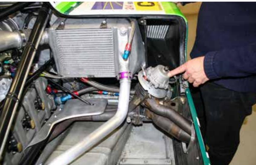
■ Detail of the turbocharger and intercooler, with stubby exhaust pipes exiting body side; these were vulnerable to side collisions.
