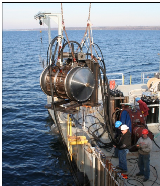
Figure 22 An early (2012) scaled-down prototype of the marine vibrator. A typical seismic array would include multiple units.
