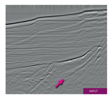
The example is a stack taken from an outer streamer, which is prone to poor/incomplete/missing image of the waterbottom given the additional crossline offset; this is shown in the change in the waterbottom character across the section. To circumvent this, the 3DSWME is fed a bathymetric surface to utilise in the 3DSWME modelling phase, to the benefit of the prediction.
