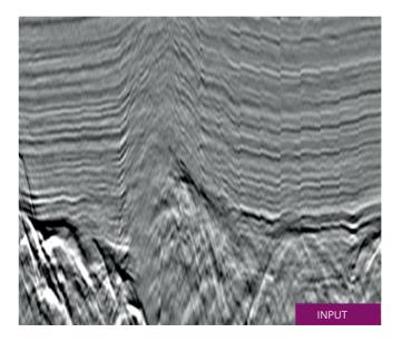
The example below shows a crossline with a clear sailline pattern highlighting the azimuthal NMO effect. The azimuthal NMO result incorporates an additional azimuth term within the NMO to account for a defined fast-slow axis.
