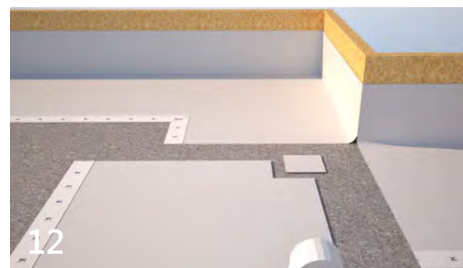
For external corners, cut a square of 403 HydroBond and from a corner of that square, cut out a small square of about 75 mm x 75 mm. Fit the square to the corner and when in place, tape the square under the 403 HydroBond already in place.
