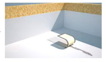
patch with HydroBond Tape, pressing firmly using a hard roller to ensure a good bond. Overseal the outer edge of the patch with Newton Mesh Tape. Use a hard roller and a heat gun to fully adhere the Mesh Tape into the membrane fleece.
